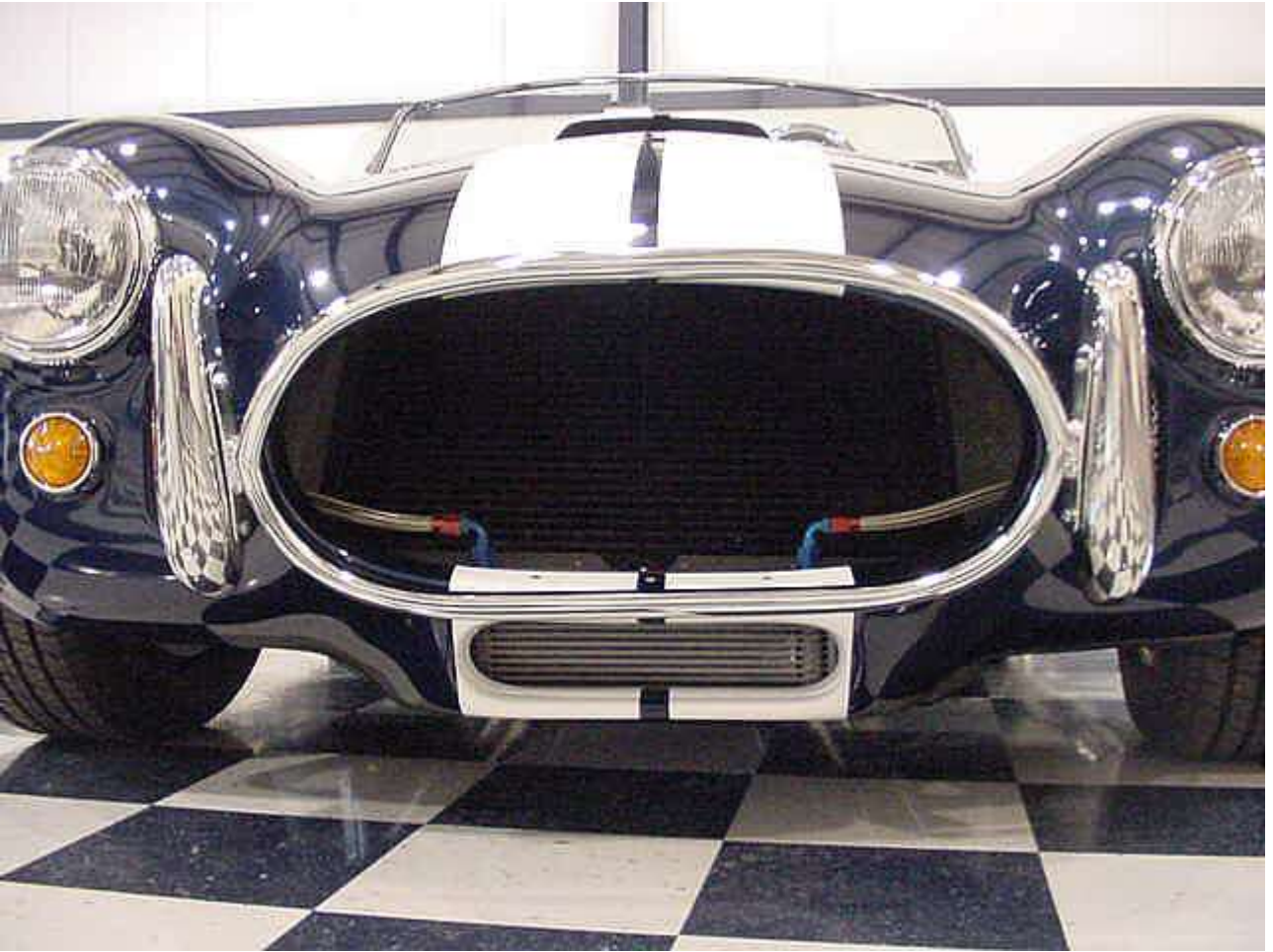
Front Overrider and Nudge bar installed.
