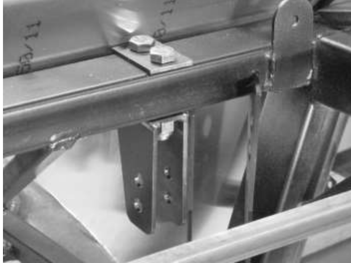
Upper mount (trunk floor not installed)
