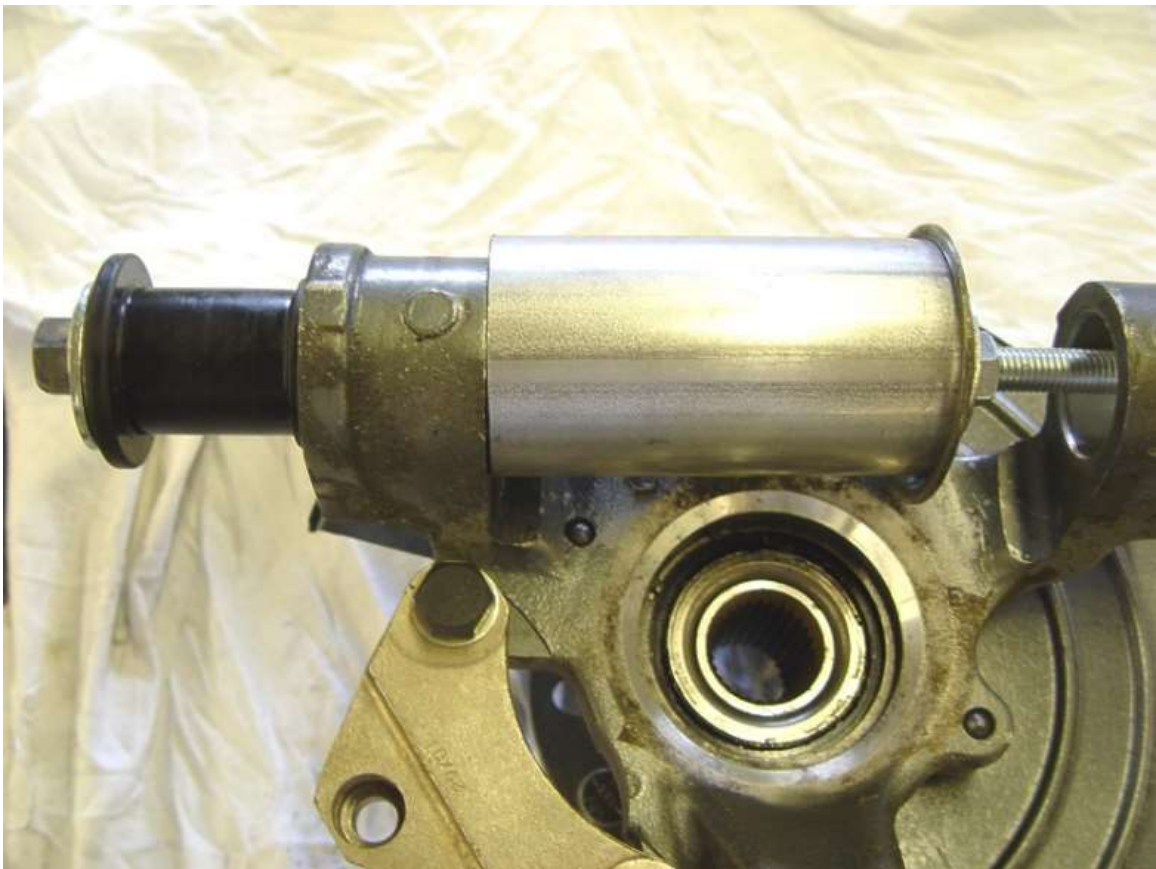
Installing a lower polyurethane bushing.
