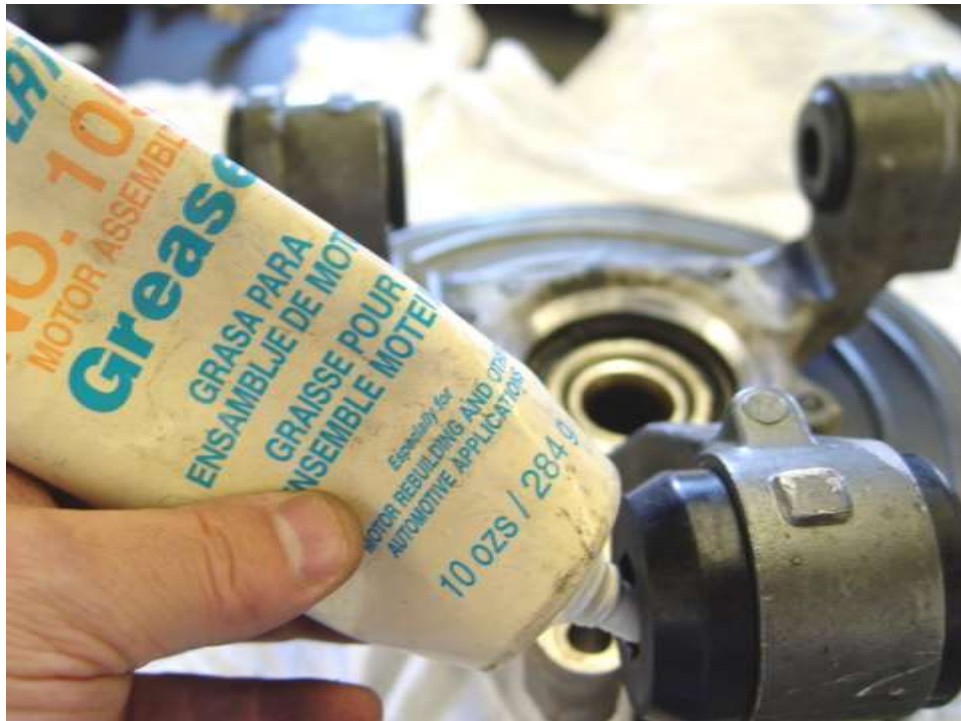
Greasing the inside of the bushing for the pivot sleeve.
