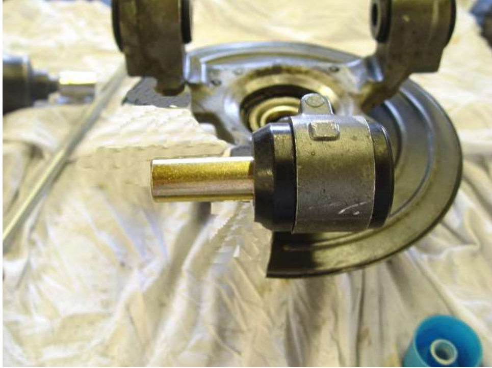
Installing the upper pivot sleeve.
