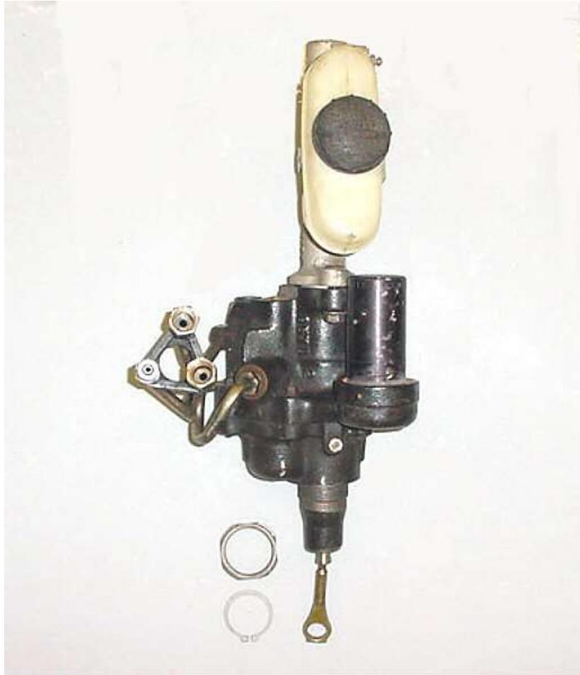
1997 Hydro-booster, Master cylinder, Hydro-booster retaining nut and snap ring.
