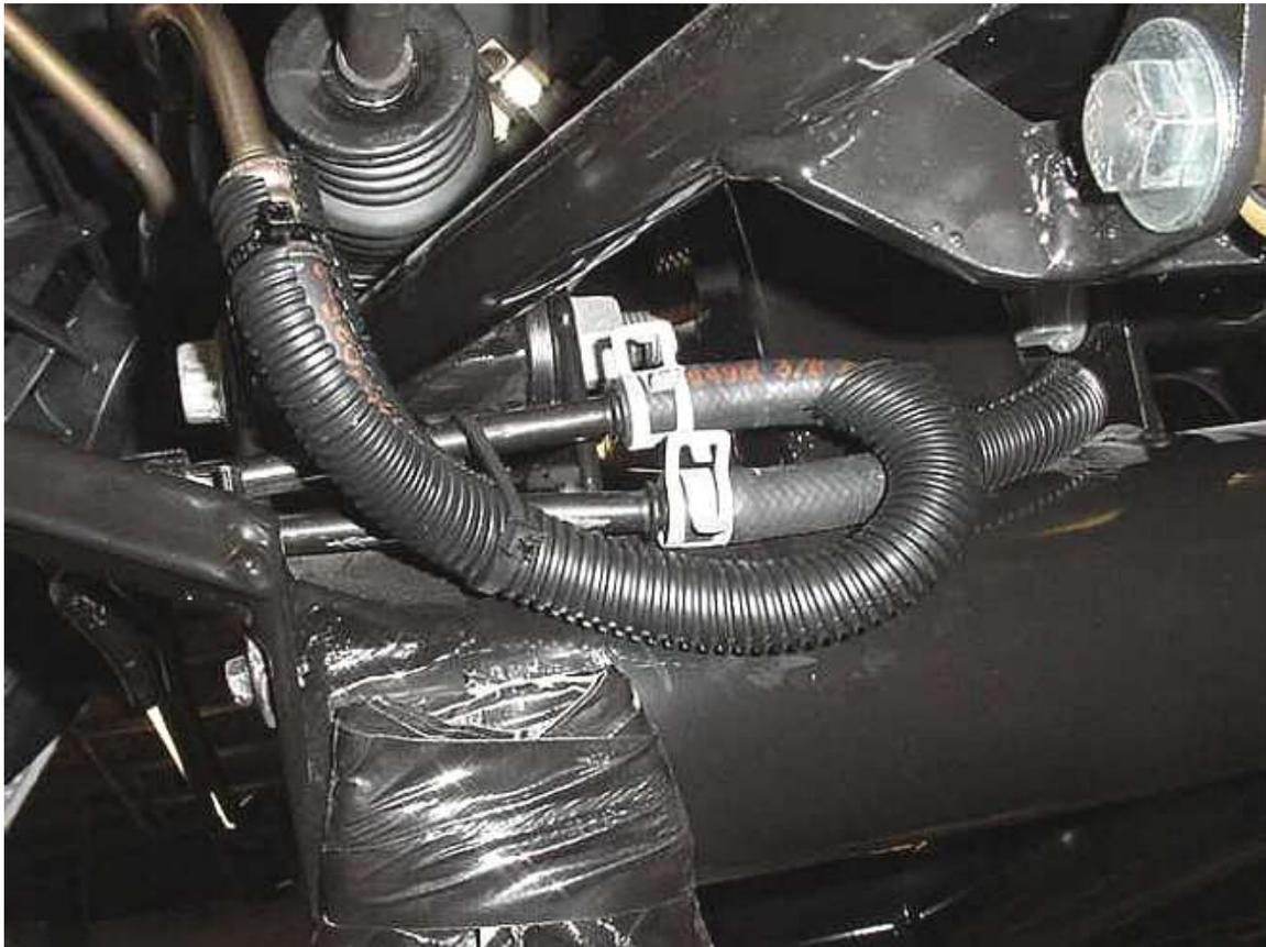
Hose routing for power steering cooler.
