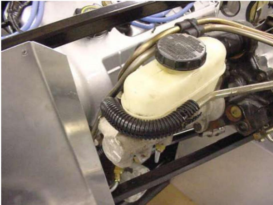
Tubes bent around inside of Master Cylinder.
