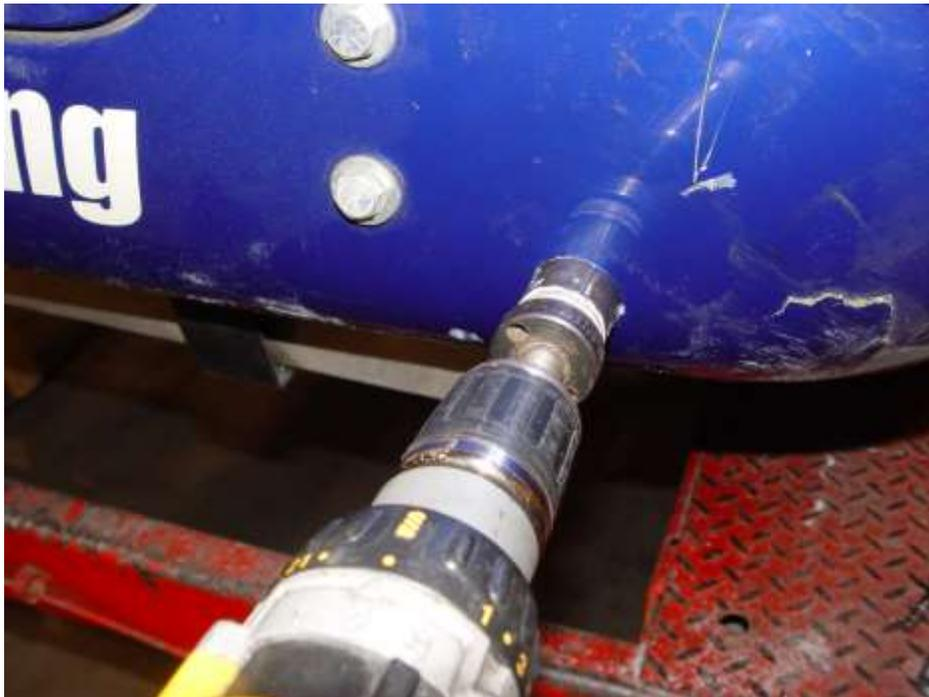
5. Drill out the chassis tube starting with small holes and progressively getting larger. Be careful with the larger sizes of bits as they can bite and catch passing through the tube. Your final hole will be  $\frac{3}{4}$ " in diameter.
