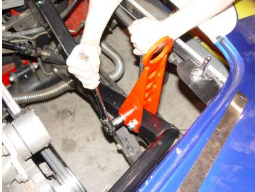
11. Set the hood back into position and fit the trim plate. It is set up for 1/8" rivets but can be screwed down to match the hood pin plates as well.
