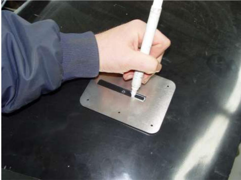
6. Drill out both ends of the slot with a  $\frac{1}{2}$ " drill and connect the two holes with your saw.
