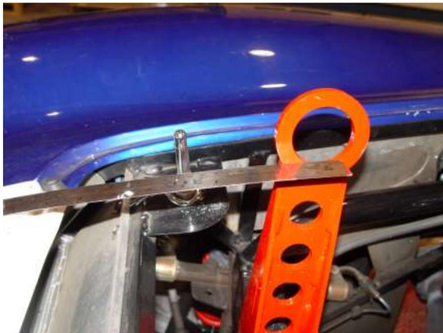
3. Once you have a height you want, clamp or tape the hook in position and put a dab of grease or anti-seize on the top.
