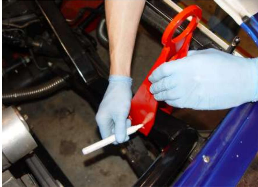
9. Remove the hook and drill the two holes. It is easier to do this if you start with small bits and work your way up. Be very careful to keep the drill straight so the bolts will fit through both sides.
