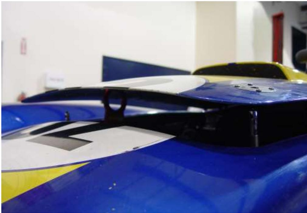
5. Drill a small hole through the hood at the center of the marked spot and then use the trim plate as a template to mark where you will cut. It is always best to start tight with the hole in case any adjustments are needed.
