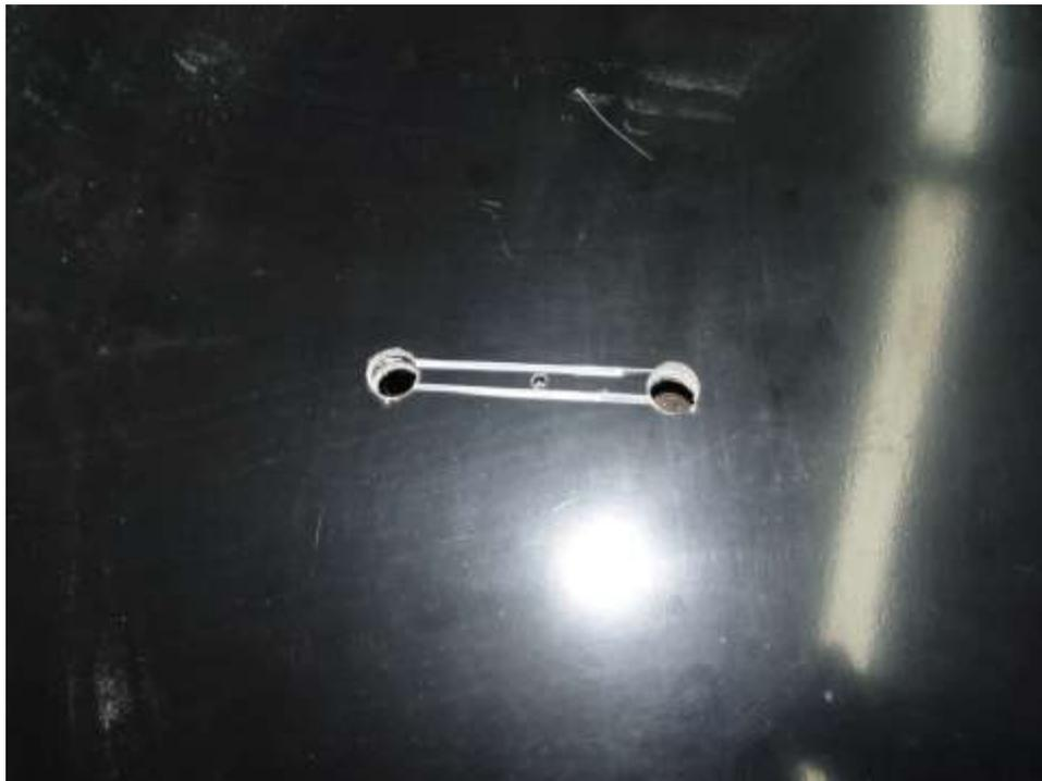
7. Set the hood back on the car and make any changes needed to the slot to get good alignment with the hook.
