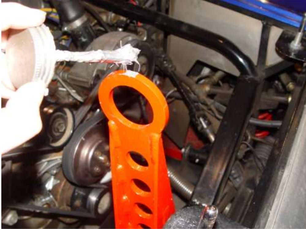
4. Gently set the hood down in place allowing the grease to mark the spot where you will need to cut the slot and then remove.
