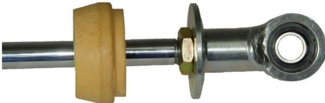
7. Put the spring on the shock, then install the spring hat on the shaft end of the shock and push the rubber bumper up against it.
