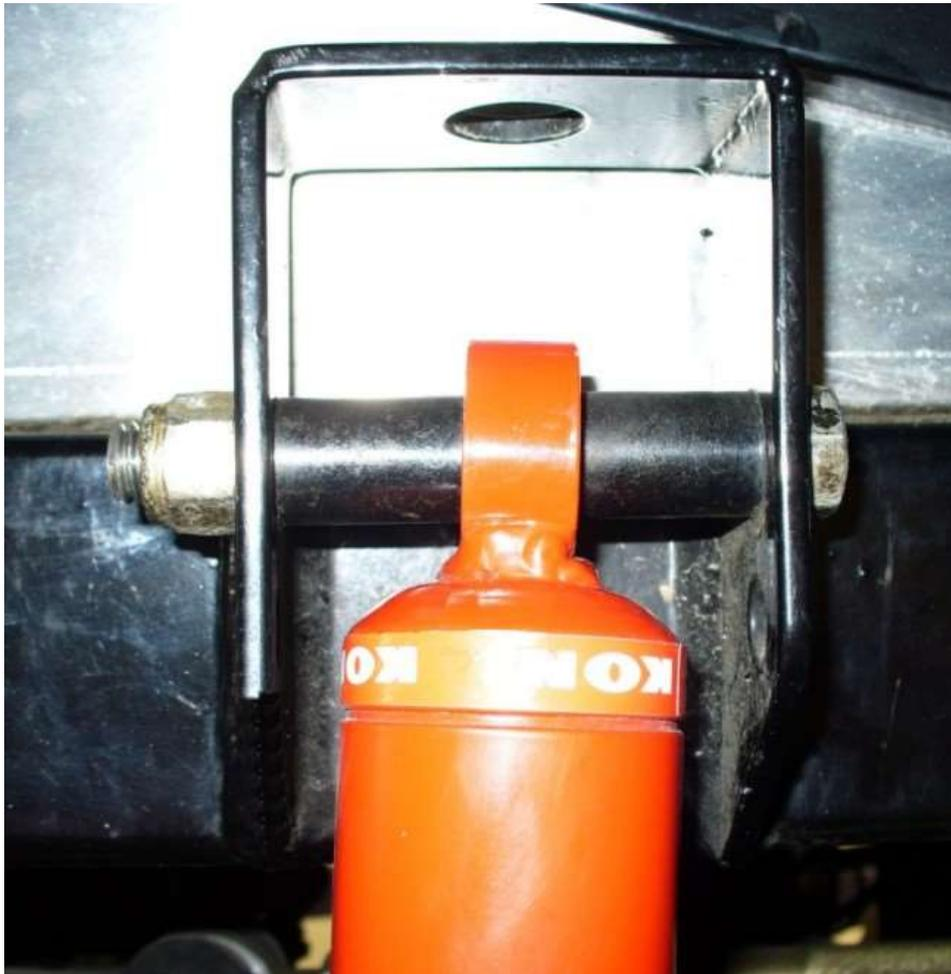
21. Install the kit  $\frac{1}{2}$ "x 4" bolt provided for the lower shock mount as was done on the passenger side. The bolt should be installed from front to rear going through the axle and bracket then the long spacer (1.13"), the shock, and the  $\frac{1}{8}$ " shim toward the rear. Once the bolt is in place with the shock and shims tighten it and the two smaller bolts that clamp the bracket to the axle. Tighten with a  $\frac{3}{4}$ " socket and wrench.
