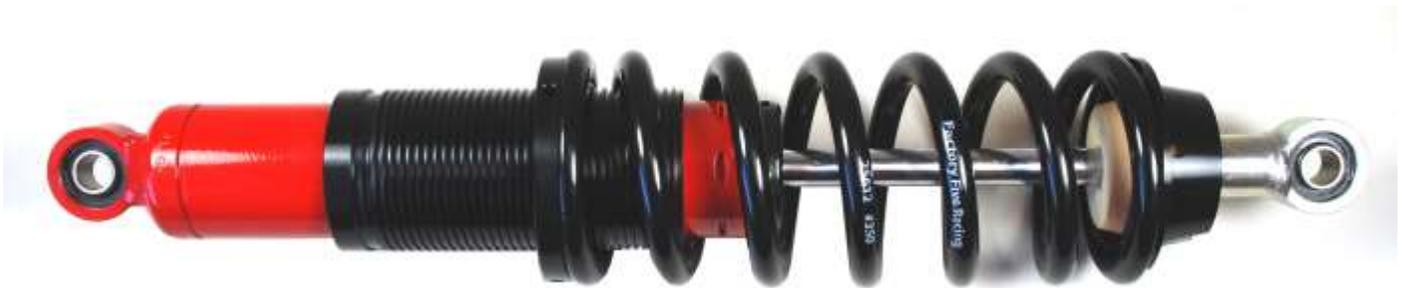
Assembled solid axle Koni coil-over shock.
