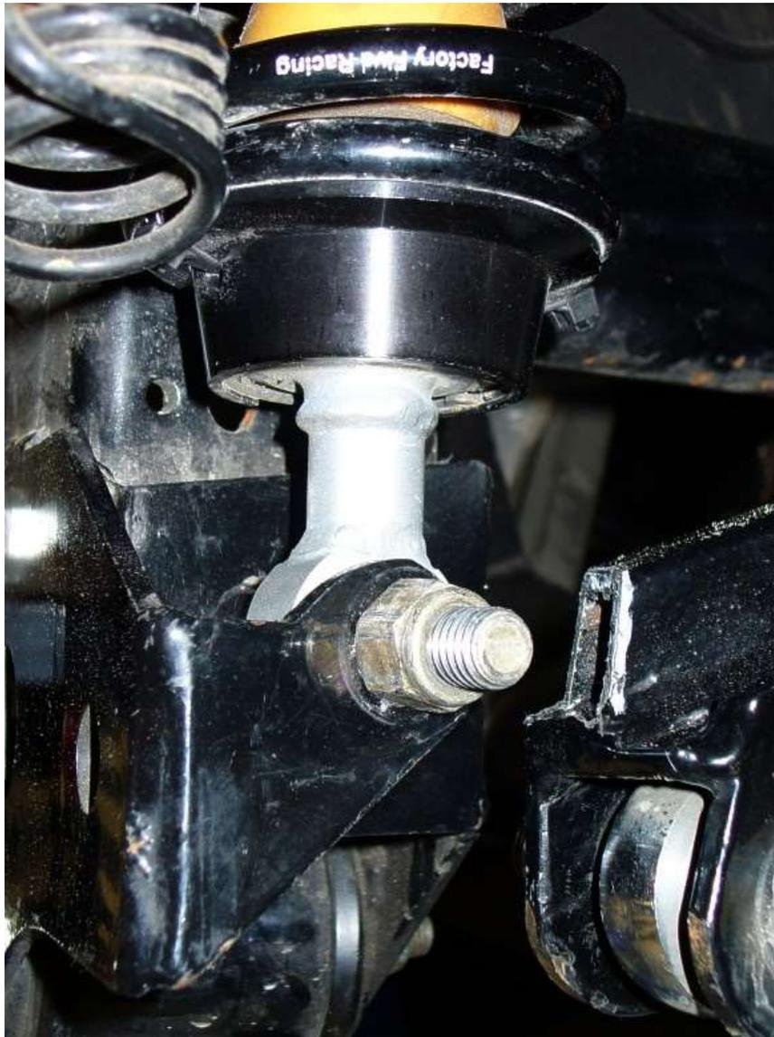
20. Install the shock by first attaching the body end of the shock to the upper shock mount using the two equal length (1.09") spacers.
