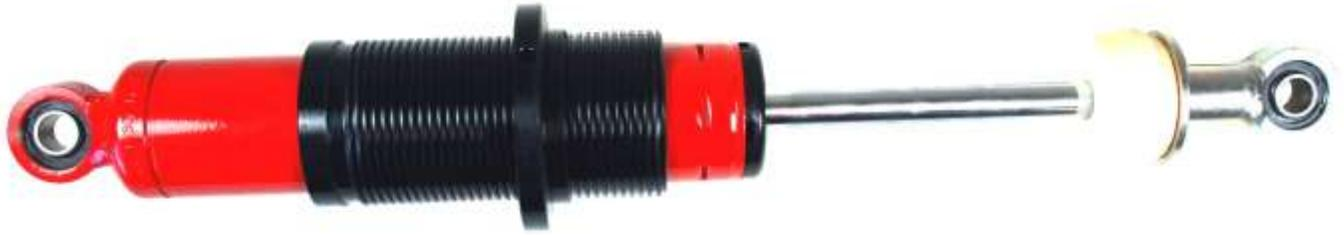
5. The coil-over hats have a snap ring which holds it in place. Remove this snap ring to assemble the coil over shock.
