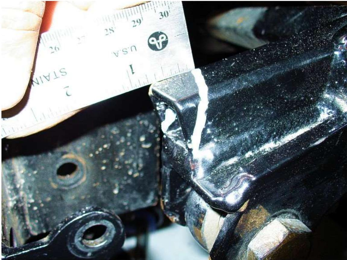
18. Cut this area off using a hack saw to allow clearance for the spring hat.
