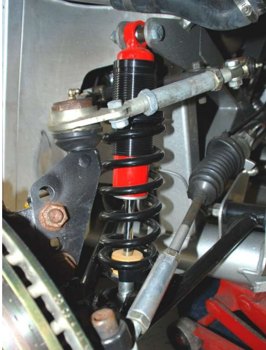
Front suspension using tubular lower control arm.
