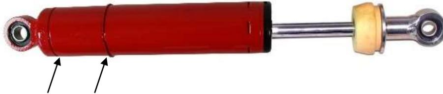
16. Once the ride height is set, tighten the small set screw in the spring seat just until you feel it contact. The end of the set screw is plastic so that the threads are not destroyed. Not a lot of pressure is needed to prevent the seat from turning.
