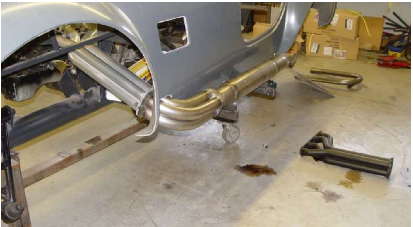
DRIVER SIDE WITH SIDE PIPE INSTALLED, FULL PROFILE
