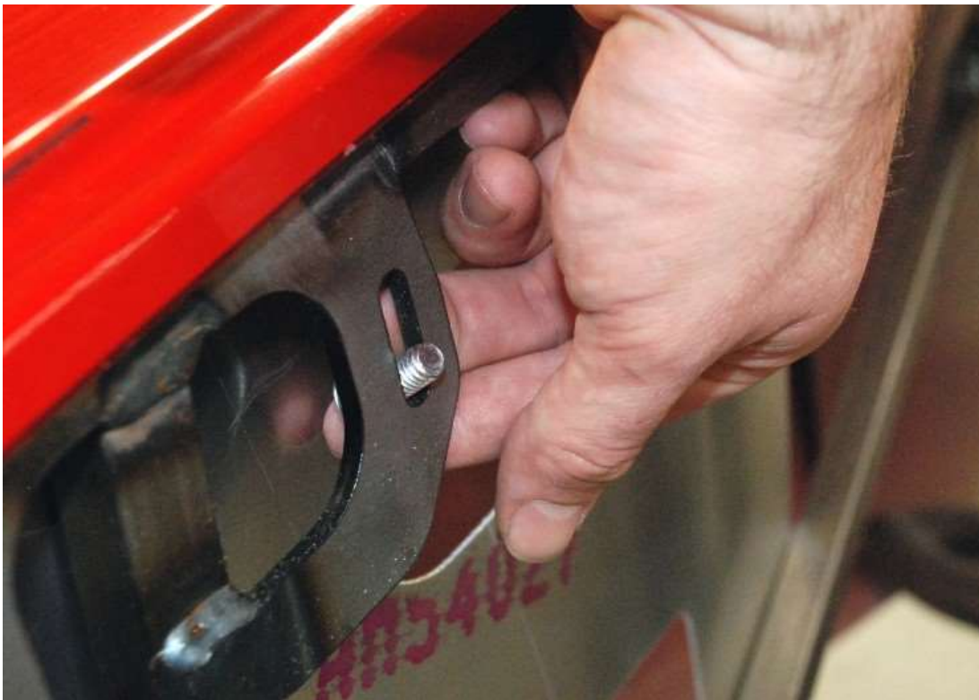
Attach the hinges to the chassis using the carriage bolts, these push in from the outside for easier adjustment.
