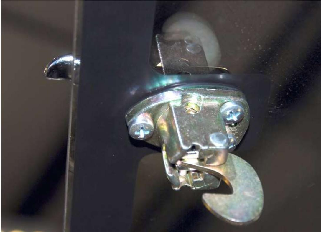
Push plastic bushings into both sides of the hatch frame hinge bracket. Use a vise to push them in evenly if necessary.
