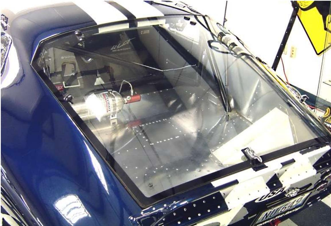
The rear hatch uses the weather stripping that has two legs on it, one longer than the other and has no adhesive on the back.
