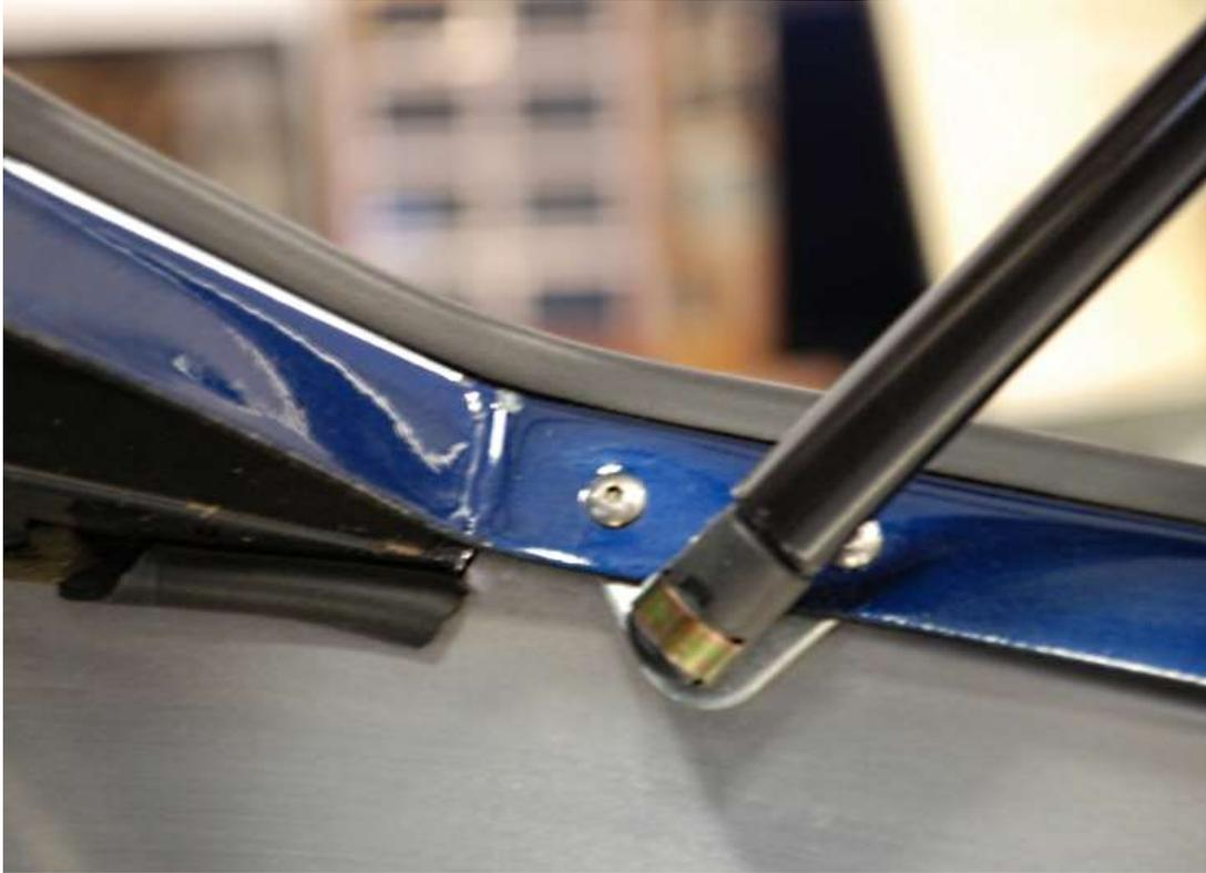
Attach the body side of the strut to the frame ball stud.
