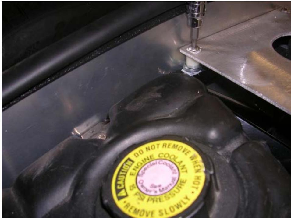
8. Screw the supplied section of threaded rod (FFR# 25723) into the rod end on the wiper motor.
