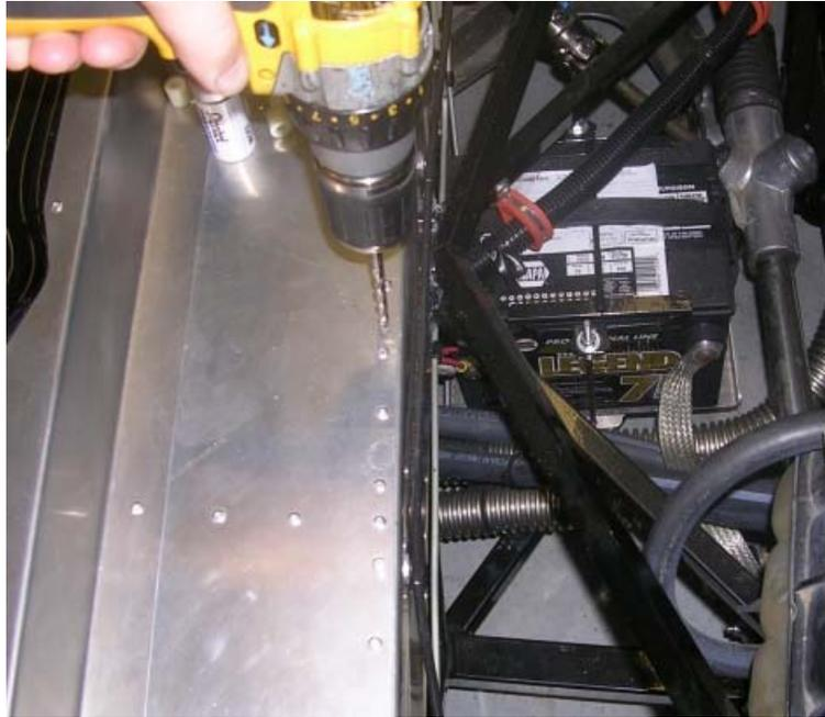
3. Install the 1/4" riv nuts (4) using the supplied riv nut tool.
