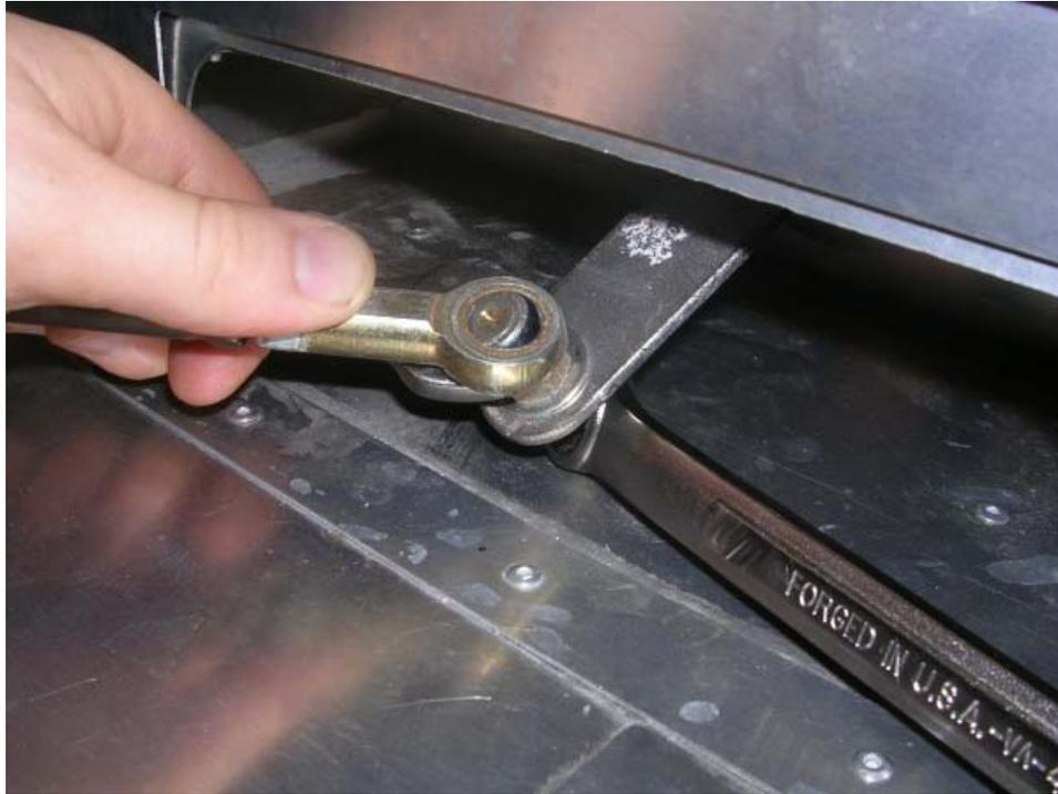
15. Install the wiper blade (FFR# 25629) onto the wiper arm (FFR# 25552).
