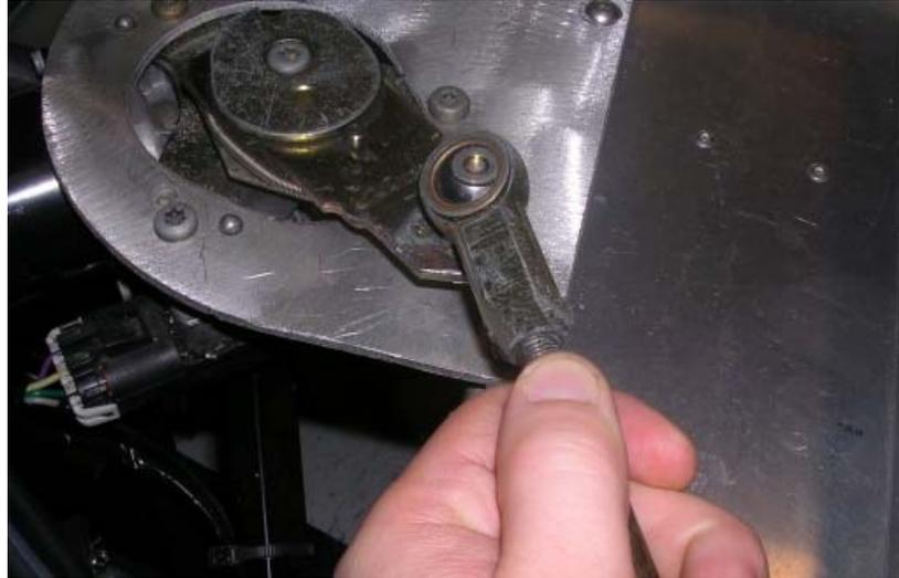
9. Slide the aluminum tube (FFR# 25934) over the threaded rod and measure how much of the aluminum tube will need to be trimmed once the rod end is screwed on. Trim the tubing with a tubing cutter/hacksaw/cutoff wheel.
