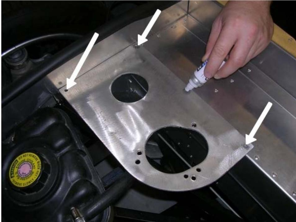
2. Drill the riv nut holes using a  $\frac{25}{64}$ " drill bit. You may want to begin by using a smaller drill bit to drill a pilot hole first (shown).
