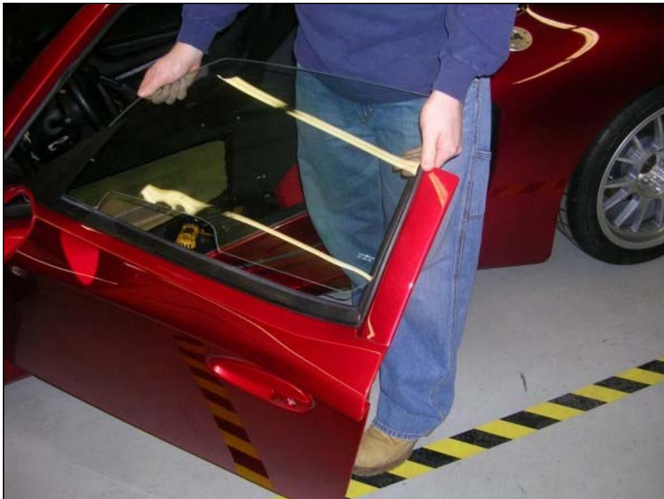
18. Set the bottom edge of the glass in the two guide clamps. Do not tighten the clamps yet.
