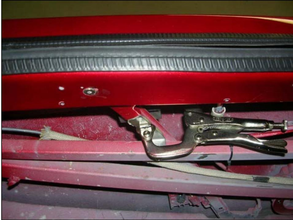
14. If you haven't done so already, install the adhesive-back weatherstrip (FFR# 12750) along the door opening on the body.
