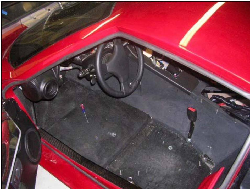
15. Using the same adhesive-back weatherstrip (FFR# 12750), install a strip along the rear door post so the bulb faces toward the front of the car. This will allow the rear edge of the glass to rest against the bulb, sealing the rear edge.
