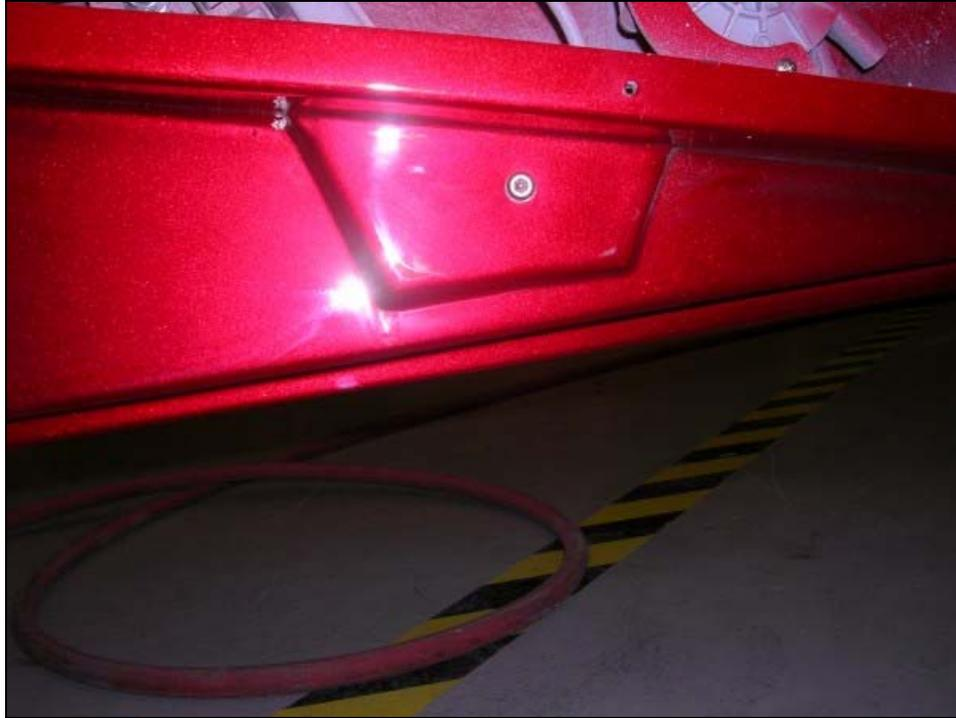
9. Adjust the tracks by pivoting them about the lower bolts. Start by positioning the rear upper track so that the bolt will be approximately 10" from the rear edge of the door and the bolt in the front track will be about 27" from the rear edge of the door.
