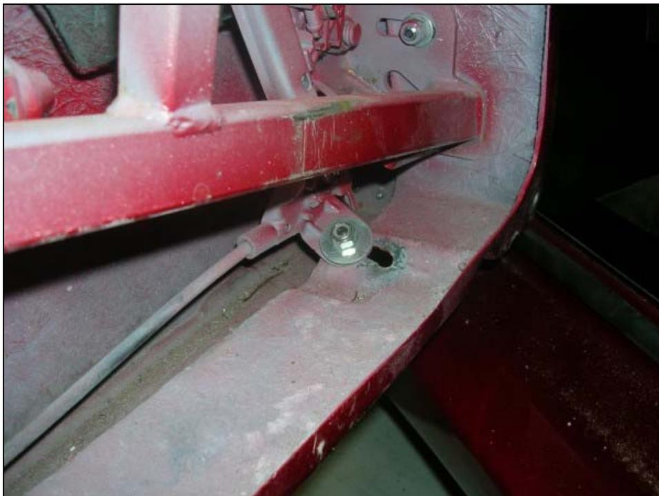
5. Place the lower portion of the rear track into the molded recess on the inside of the door near the back of the door.
