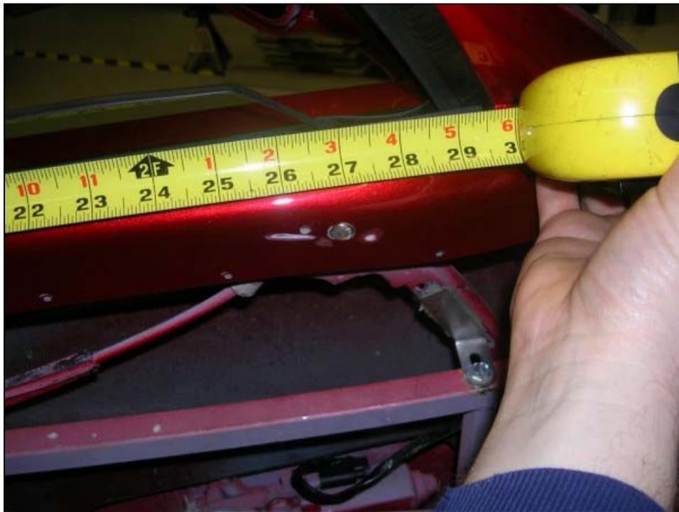
10. Before mounting the Window Track Brackets (FFR# 25859, 25860), notice that the brackets should rest against the window track, and sit flat against the top edge of the door frame (shown bonded and bolted in place).
