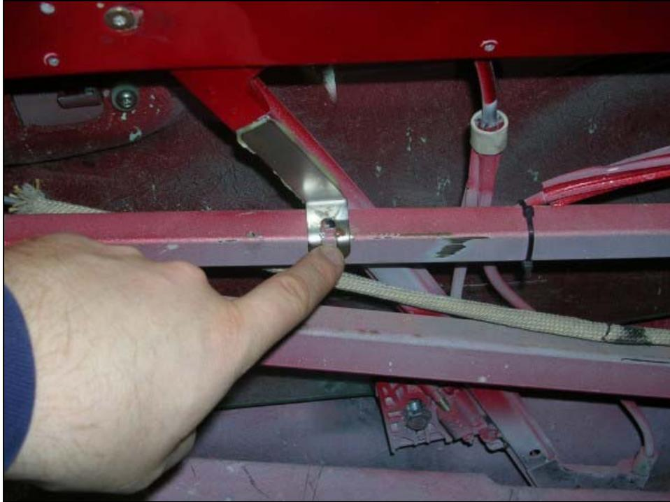
21. Once you are sure the window will move freely, tighten the window tracks and the guide clamps to the window.
