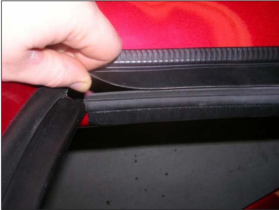
17. Slide the glass through the slot in the top of the door.
