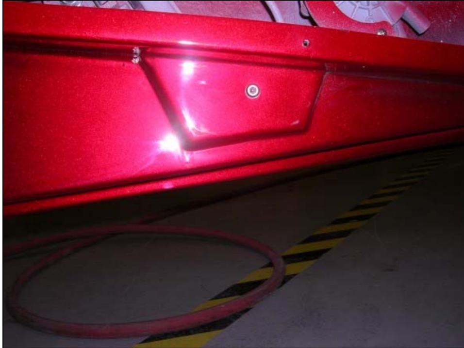
7. Drill a 6 mm (approx 1/4" if you don't have a 6 mm drill bit) hole in the door pocket.
