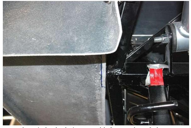
If necessary cut the running board so that it goes around the frame near the rear fender.
