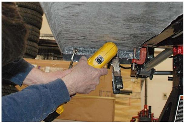
Drill 1/4" mounting holes through the rear lip of the running board into the rear fender.
