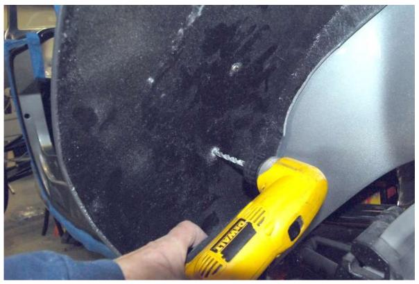
Drill a <sup>3</sup>/<sub>16</sub>" hole straight up making sure it goes through the rear fender and the body.
