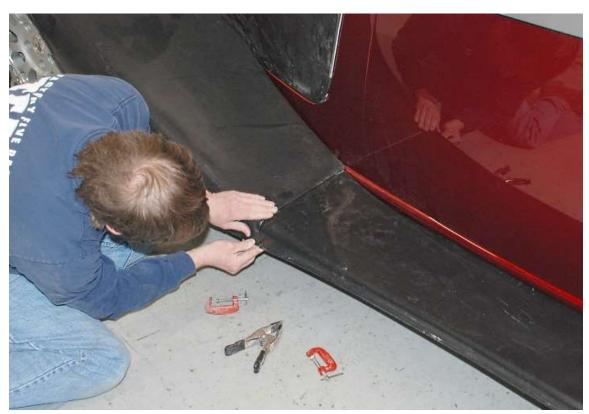
Put the front fender on over the wheel and then align and clamp it to the front of the running board.
