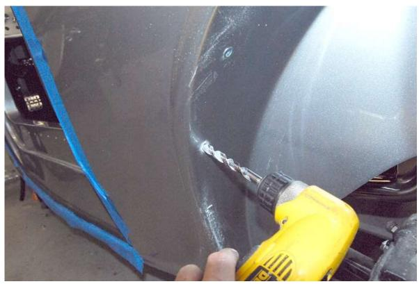
Remove the fender and enlarge the hole in the body to <sup>25</sup>/<sub>64</sub>"
