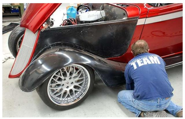
Locate the fender over the wheel while the front is at ride height to allow for 2.50" of wheel travel up and draw a line on the engine side cover.
