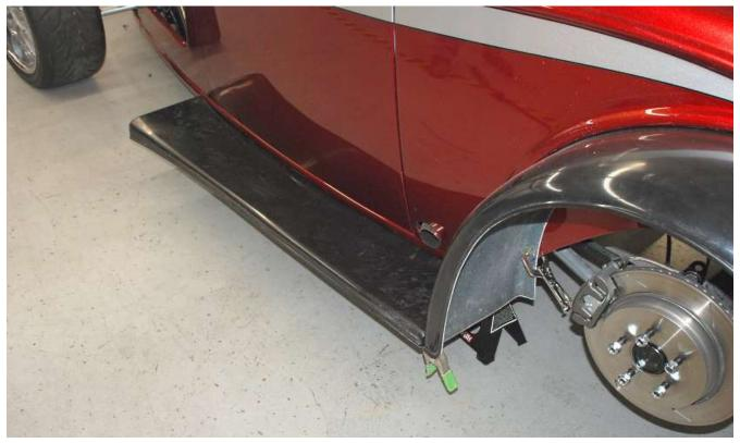
Clamp the running board to the rear fender. If necessary rotate the fender so that the fender is horizontal and lines up with the body.
