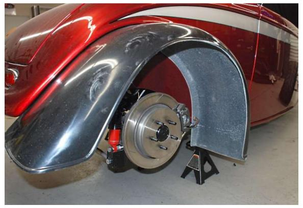
Position the rear fender on the body so it fits tight on the inside, hold it in place with clamps.
