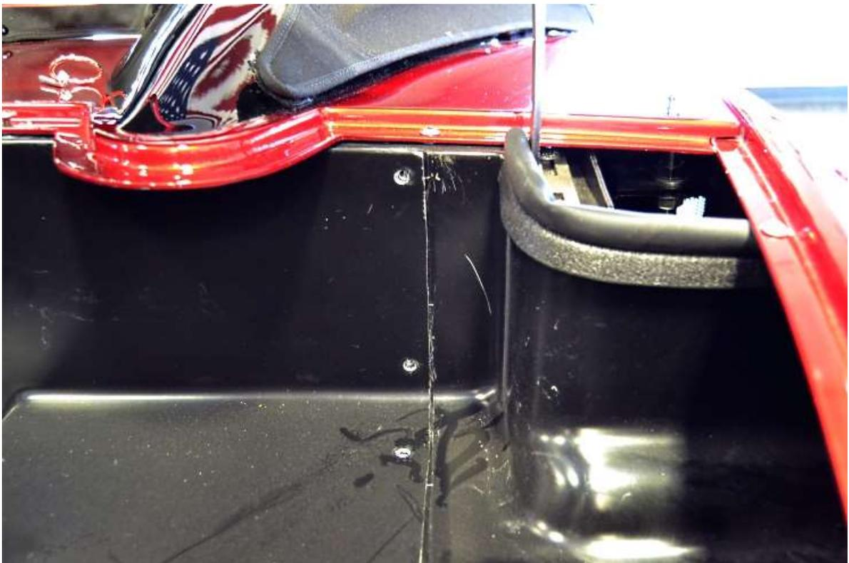
Insert the middle trunk panel so that the front and rear flanges are under the body flanges like the side panels then tighten the side trunk panel screws.
