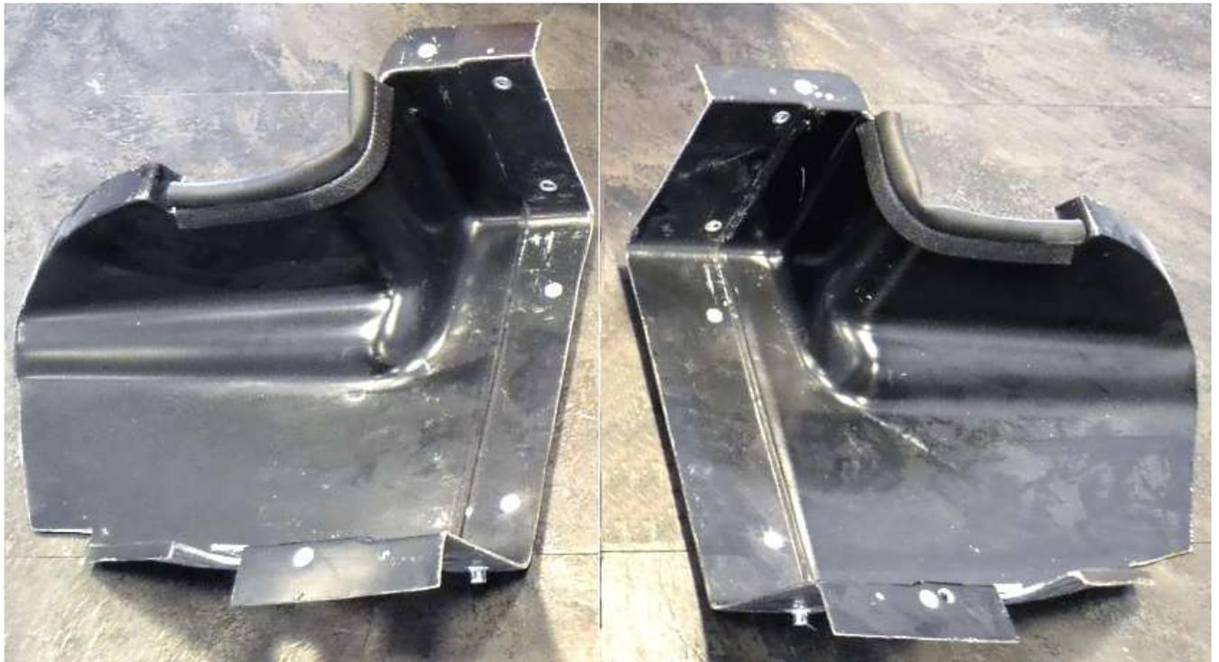
On the left and right trunk panels at the  $\frac{1}{8}$ " hole locations, drill the holes out using a  $\frac{25}{64}$ " drill bit and install rivnuts.
