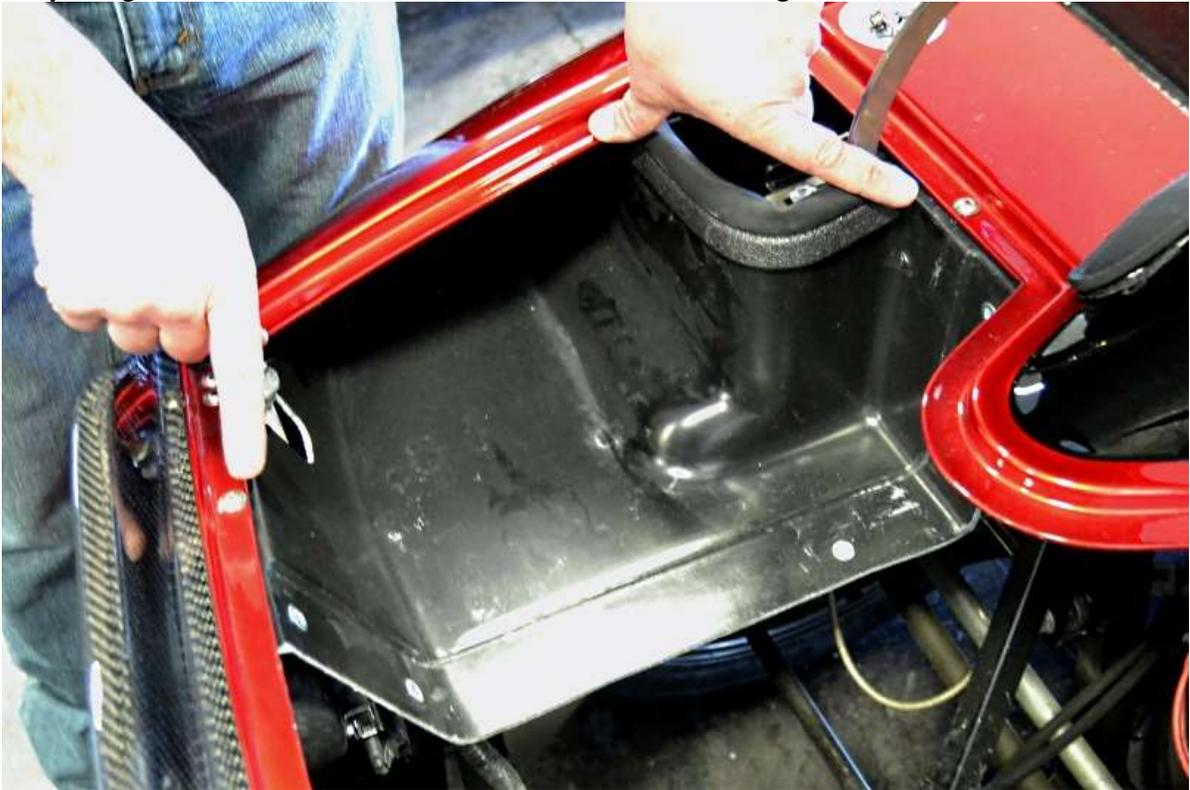
Reinstall the trunk side panels and fasten to the body flanges using the  $\frac{1}{4}$ " x  $\frac{3}{4}$ " flange head screws but do not tighten them yet.
