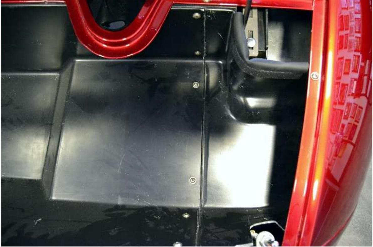
Drill  $\frac{1}{8}$ " pilot holes through each side of the trunk, (2) on the front face, (2) on the bottom face and (2) on the rear face.
