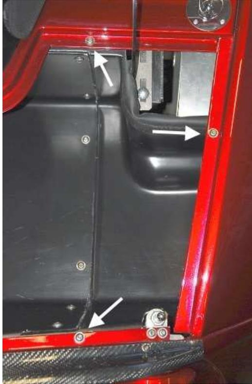
Use an  $\frac{1}{8}$ " drill bit to drill (3) bolt locations through both the body flanges and the trunk flange.
