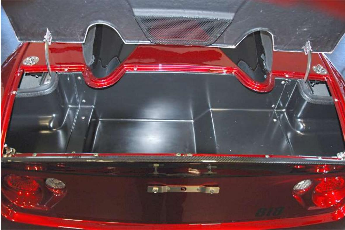
Reinstall the center trunk panel using the remaining  $\frac{1}{4}$ " x  $\frac{3}{4}$ " flange head screws.
