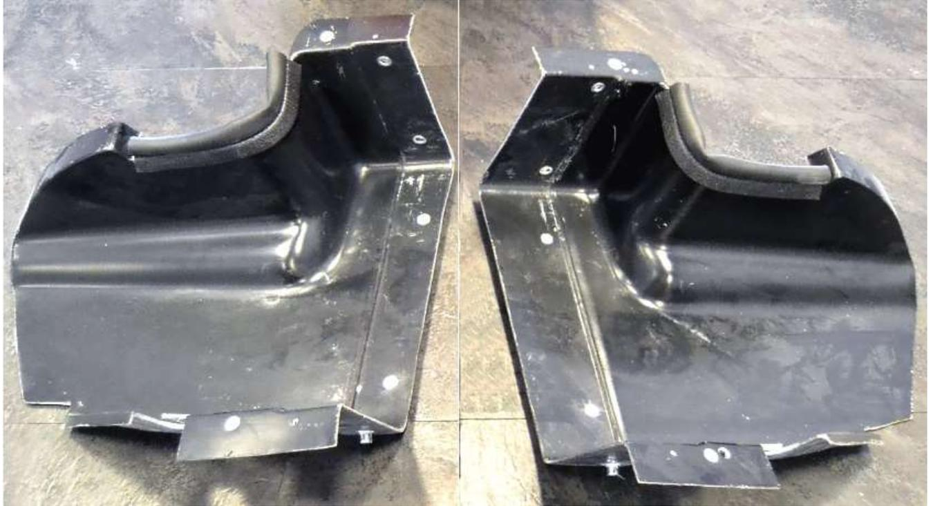
Cut the weatherstrip into (2) 6" pieces and push onto the front corners of the trunk parts.
